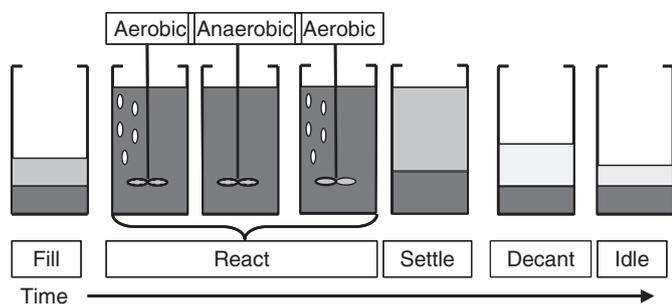
Fig. 1. Typical sequencing batch reactor operation.
