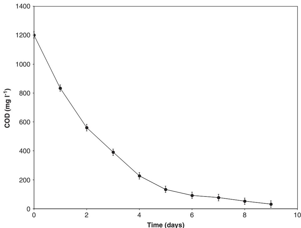
Fig. 3. COD of wastewater sludge SBR during operation of SBR for 8 days. Results are mean values for four reactors  $\pm$ SD.
