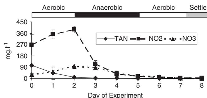
Fig. 2. Concentration of ammonia (TAN), nitrate (NO<sub>3</sub>) and nitrite (NO<sub>2</sub>) in wastewater sludge during operation of SBR for 8 days. Results are mean values for four reactors ± SD.
